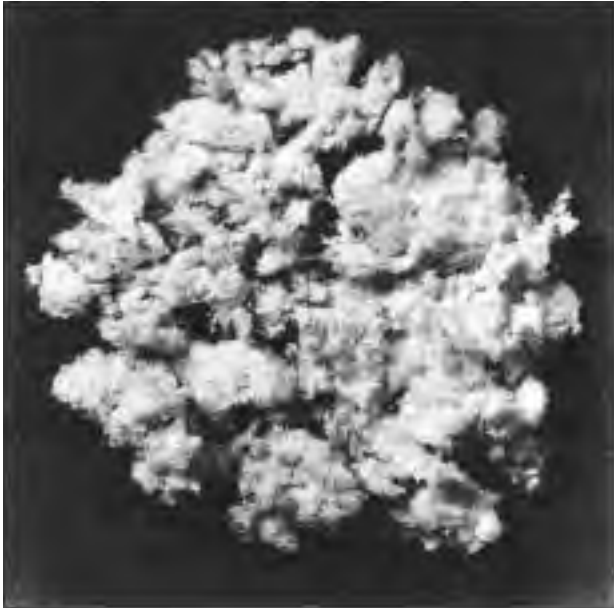
Figure 3.2 Photomicrograph of Kevlar® Pulp.
