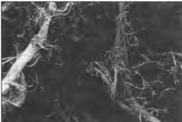
Figure 3.2 Photomicrograph of Kevlar® Pulp.
